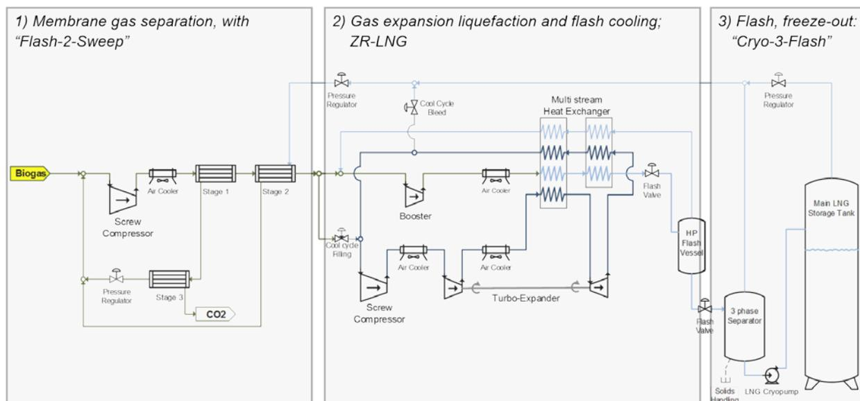
Figure 1; ZR-iLNG process scheme for biogas applications
